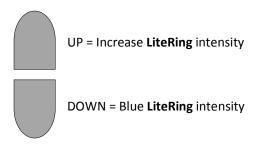
The light output can be very finely controlled in 256 discreet steps (i.e. values of 0 to 255).
