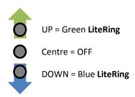
Note – The controller will remember the last dimmer setting for the Blue & Green channels independently, even when disconnected from the power source, to allow the user fast set up and change over between **LiteRing** colours.
